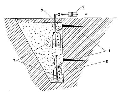
Figure 2. Installation of the lysimeters in soil [6].
